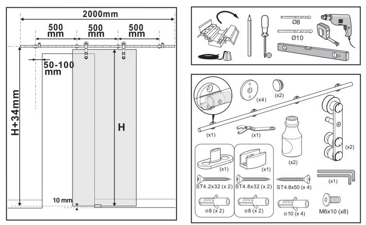
To obtain the maximum weight capacity, all fasteners must be mounted securely into solid wood of studs or blocking within the wall or wood mounted to the face of the wall.
